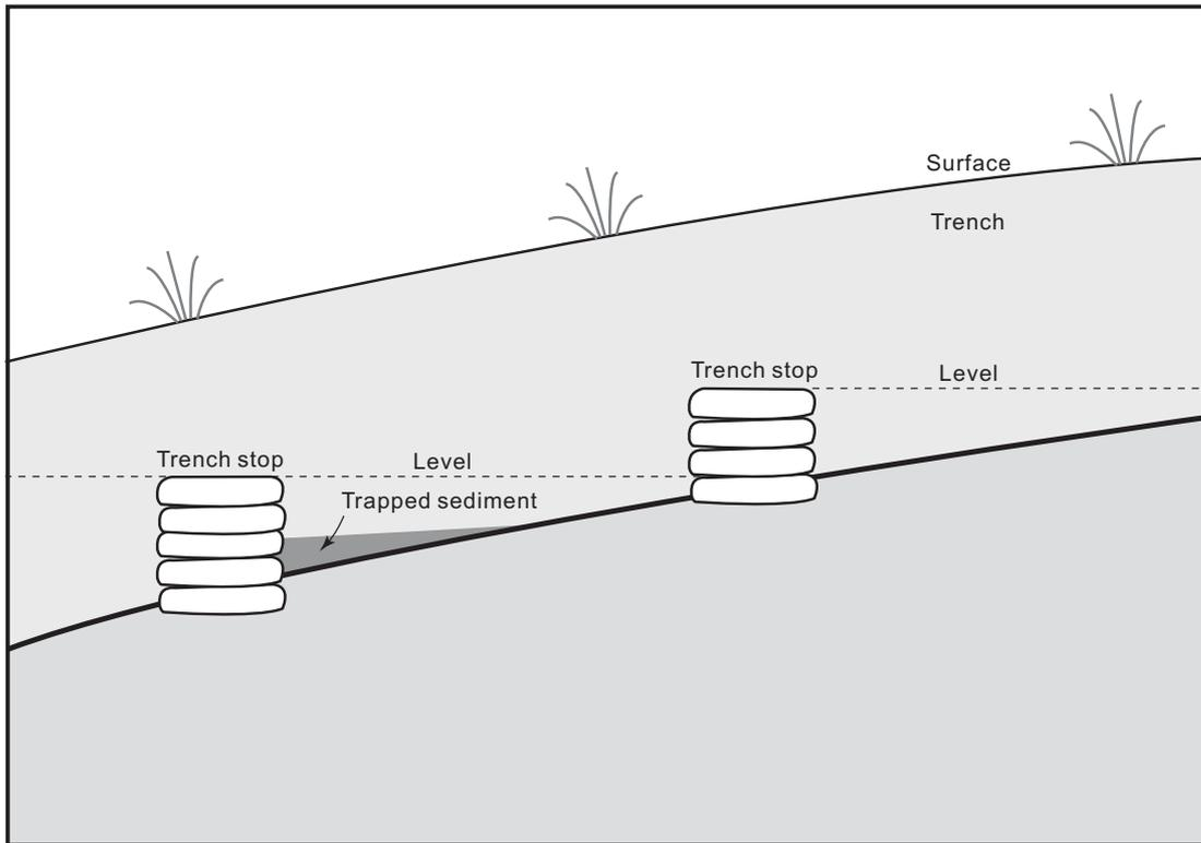
**Figure 6.2 Typical trench stop detail**
