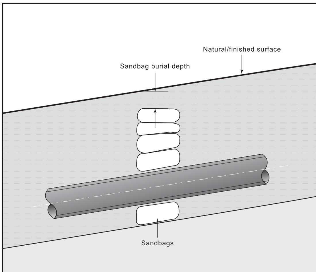
**Figure 6.3 Detail of typical seepage collar or bulkhead**
