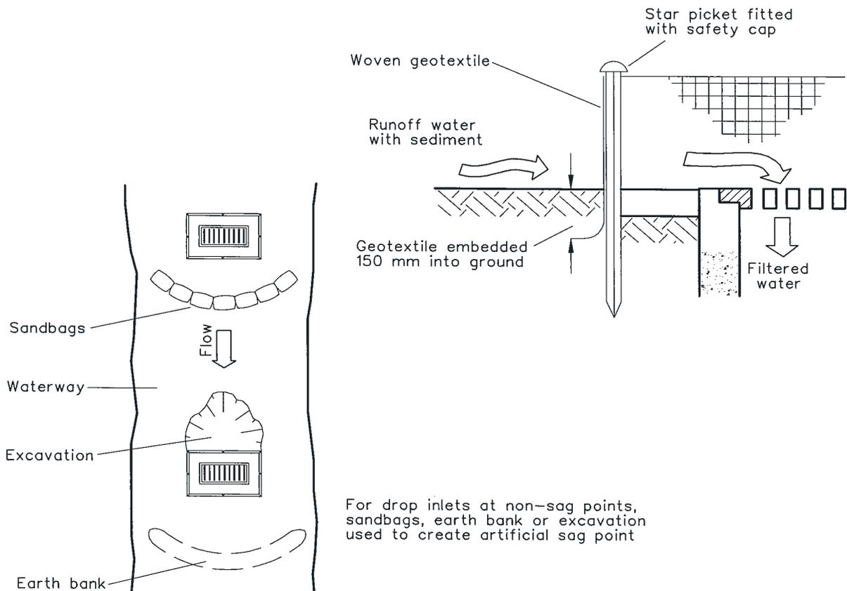
For drop inlets at non-sag points, sandbags, earth bank or excavation used to create artificial sag point
