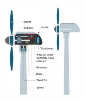
**Figure 3-1 Wind Turbine Components**
