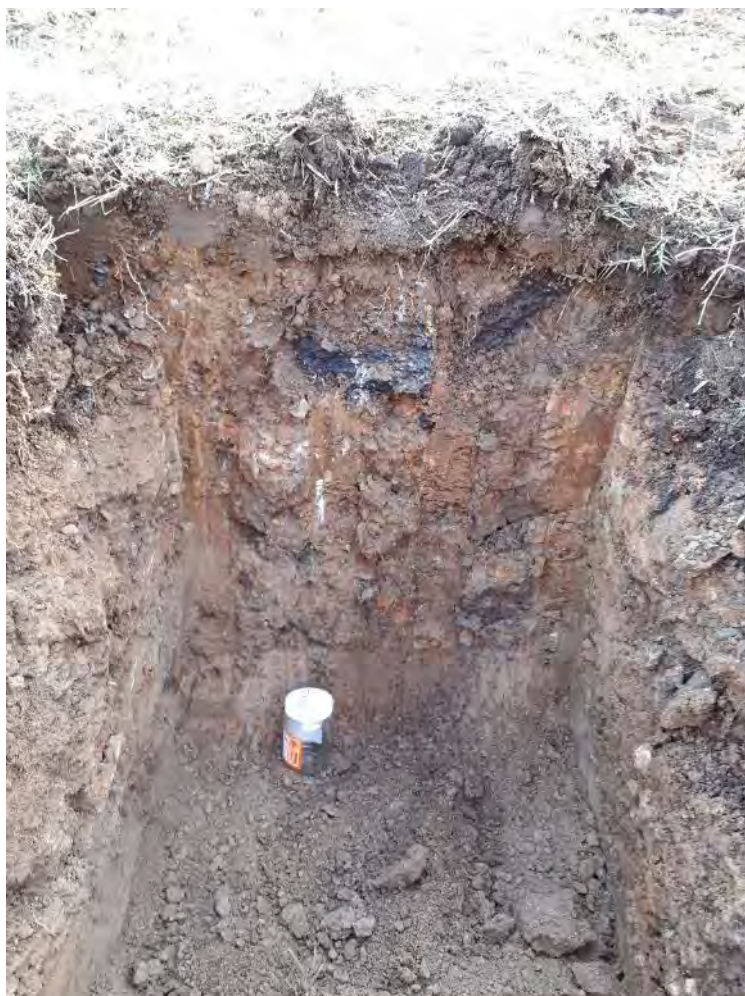
Plate 12 – Profile of STP4 dug into area of uncontrolled fill
