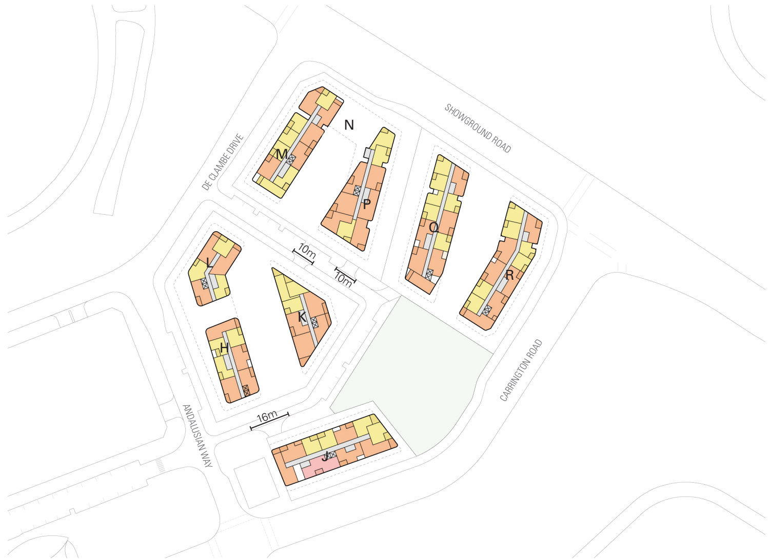
Figure 103: Precinct East Typical Level 04/05/06 - Apartment Mix
