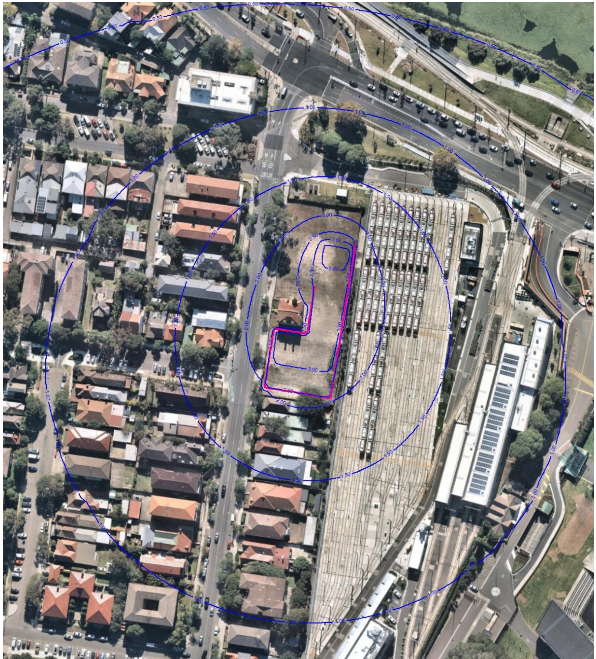
Figure 3 – Simulated Groundwater Drawdown Levels During Temporary Dewatering
