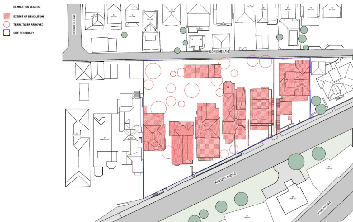
Figure 11 Extract of Demolition Plan.
