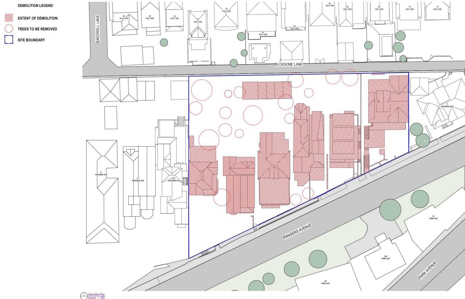
Figure 2: Proposed works – Demolition plan
