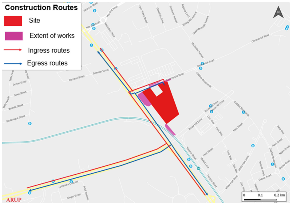
Figure 30: Heavy vehicle access routes (after completion of upgrade of Commercial Road / Health Co access intersection)
