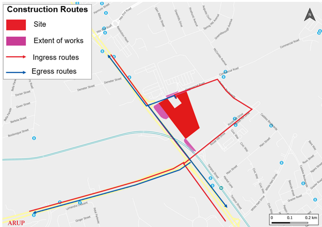
Figure 29: Heavy vehicle access routes (prior to completion of upgrade of Commercial Road / Health Co access intersection)
