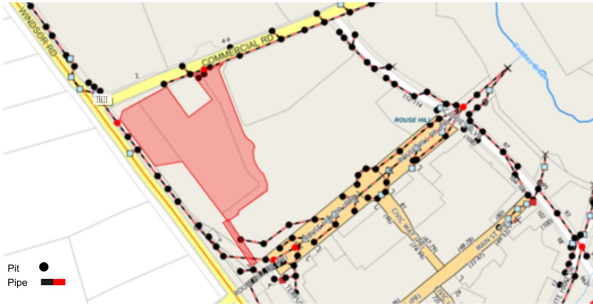
Figure 1: Existing Stormwater Network (Extracted from DBYD)
