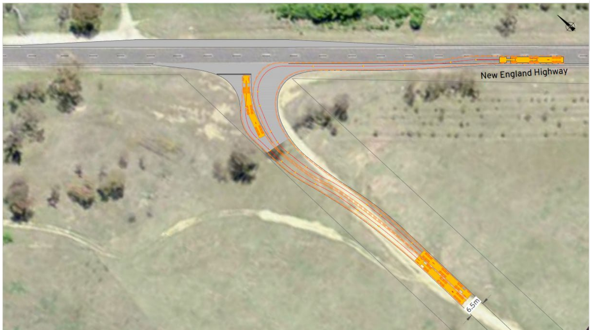
Figure 4-5 Amended intersection showing B-double engagement
