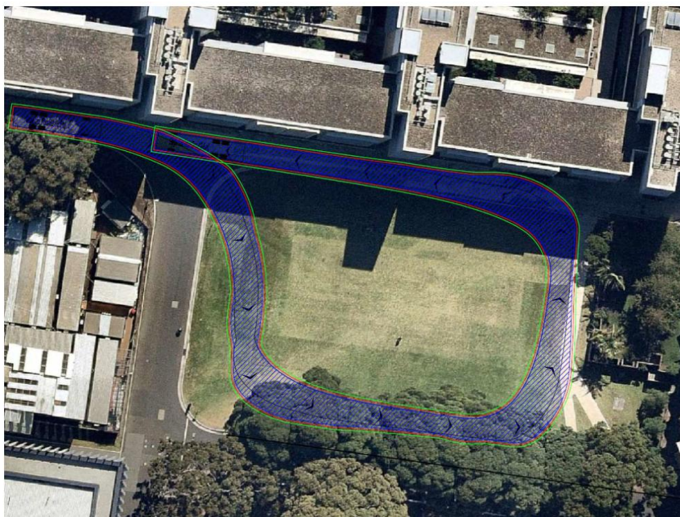
Figure 3 Swept path Analysis - site circulation loop
