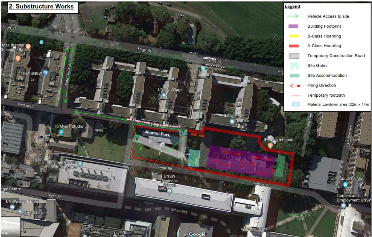
Figure 6 Substructure works & Piling works
