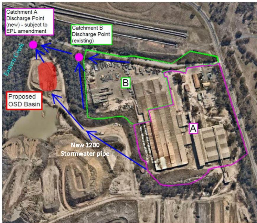
Figure 10-5 – AT&L SWMP and Civil Engineering Design Report (March 2020) Figure 4 Proposed Catchments A and B as they will be divided when the full area of Stage 2 has been developed. During the early parts of Stage 2 there will be a gradual transition from the Stage 1B catchments to the Stage 2 catchments.
