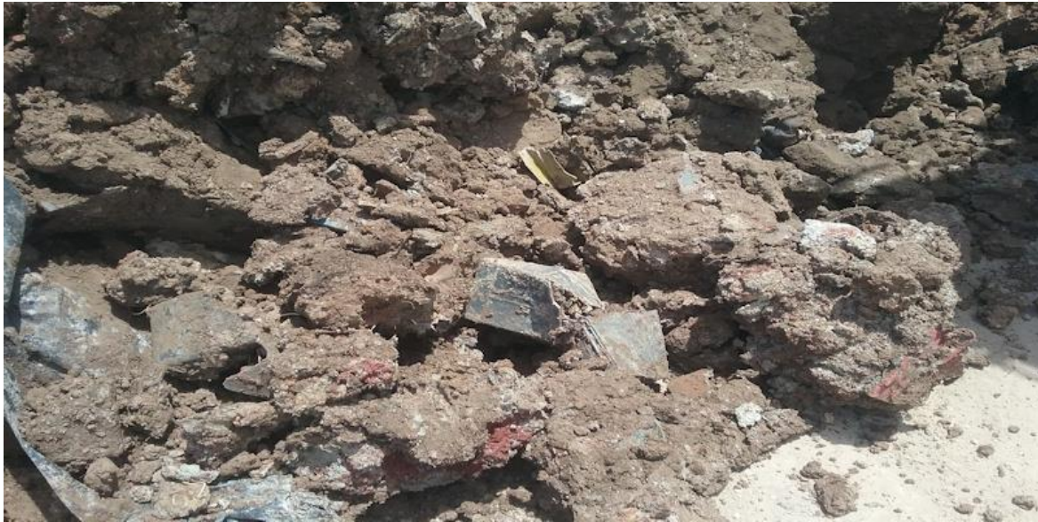
Figure A9 – This soil is bound together in an unusual way indicating that perhaps some liquid was dumped with the plastic and metal pieces that can be seen .
