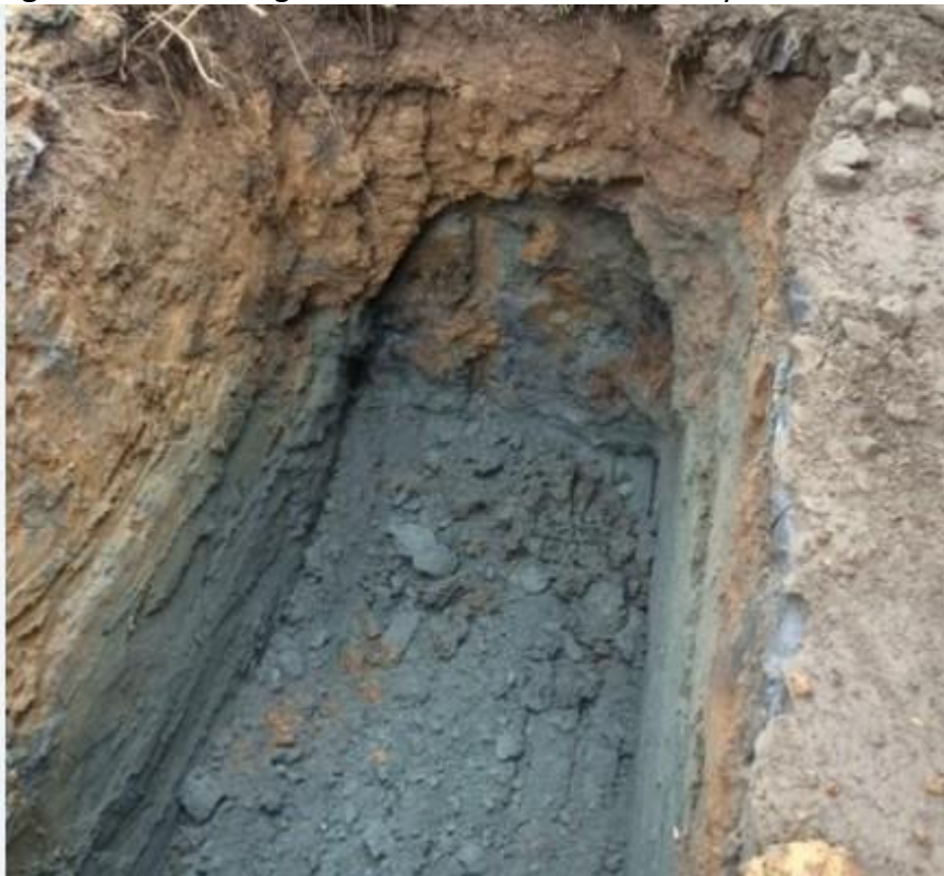
Figure A2 – Differing colours and texture of soil at depth may indicate contamination
