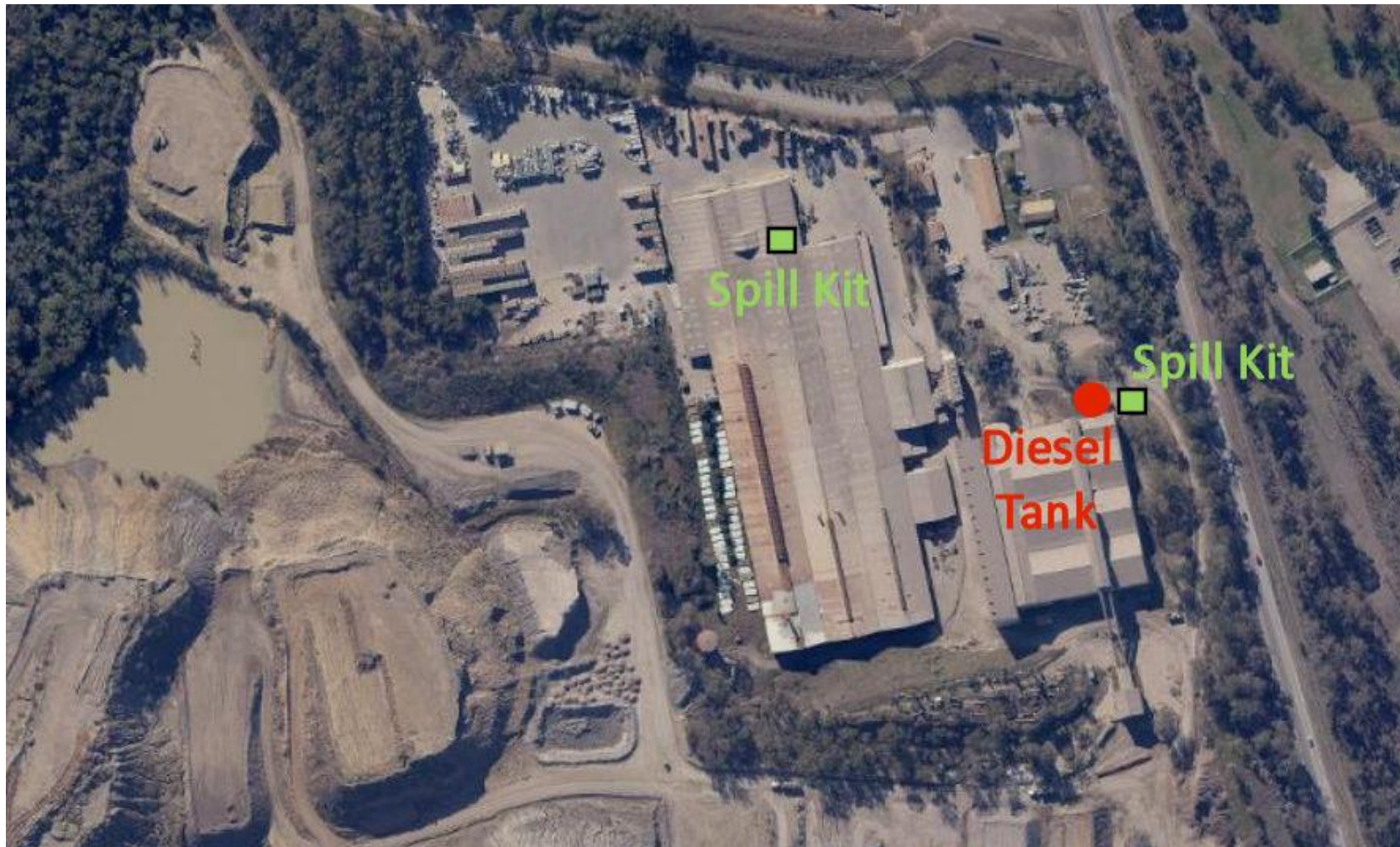
Figure 15-1 – Site Plan of Plant 2 prior to the upgrade commencement showing Spill Kit locations and the location of the Diesel Tank. The Spill Kit locations will probably be moved at different stages of the demolition and construction.
