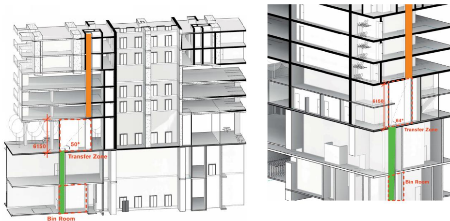
Figure 9: Angles between residential and podium chutes for North (left) and South (right) towers
