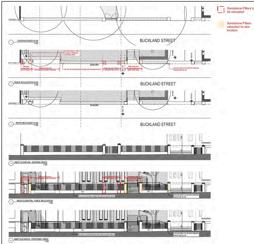
Figure 6. Heritage Fence Works
