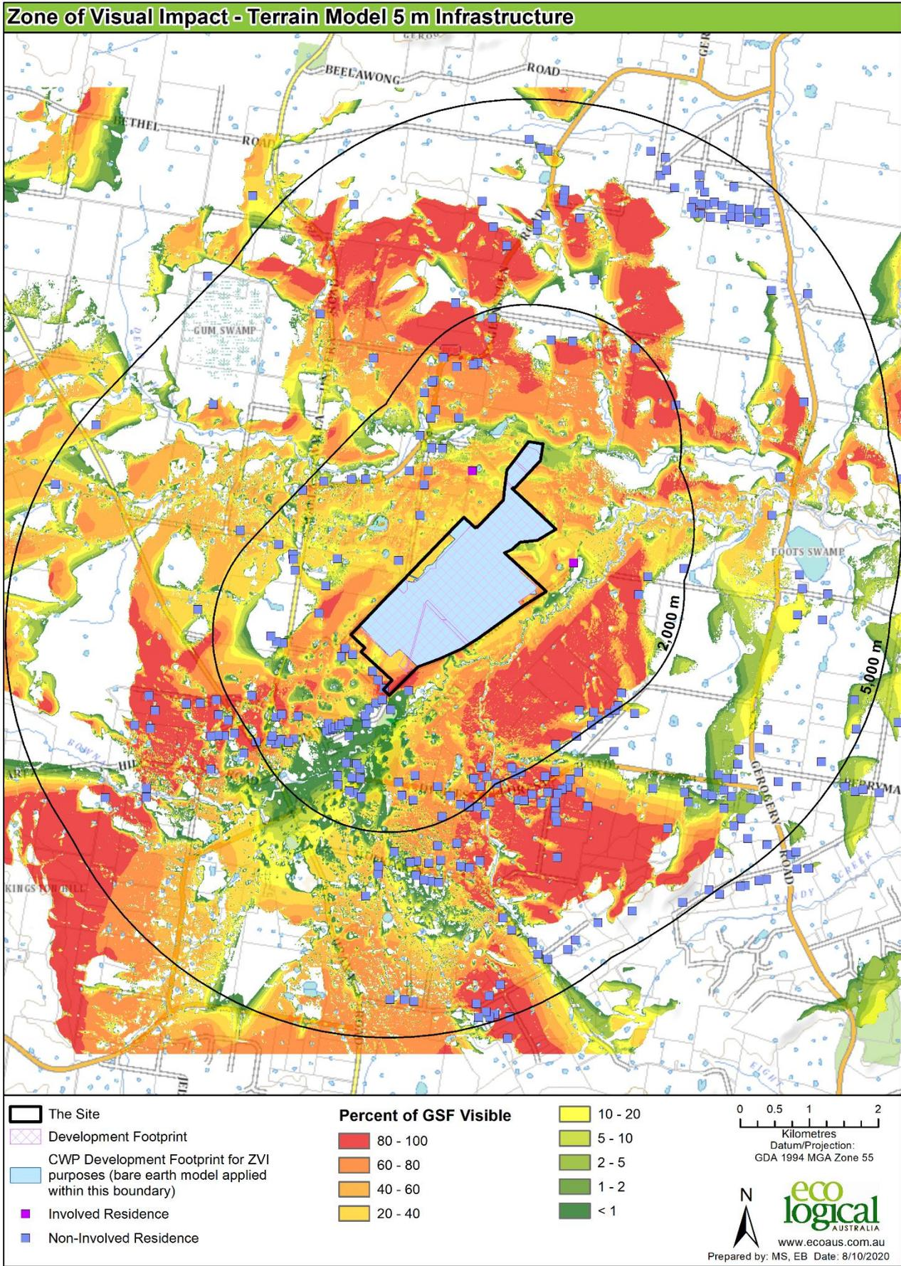
Figure 8-16: Bare earth ZVI for 5 m tall panel array
