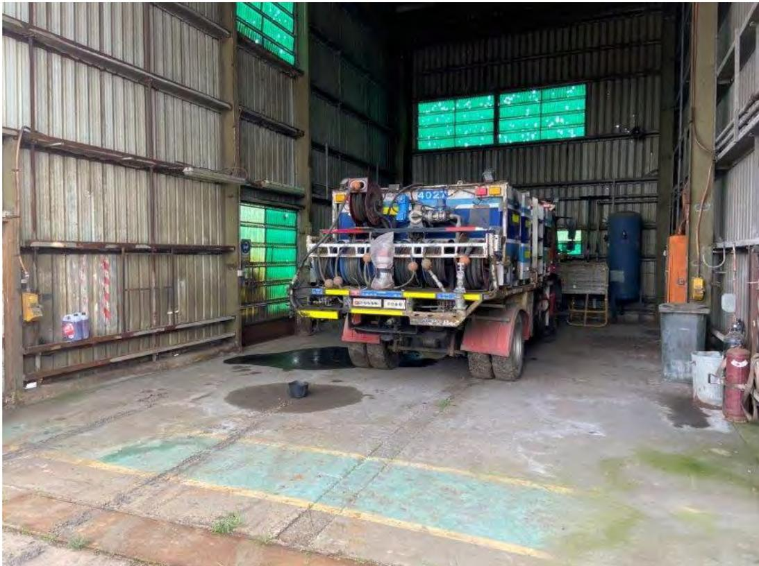
Plate 26 – Fuel and oil leaking from fuel cart during site inspection
