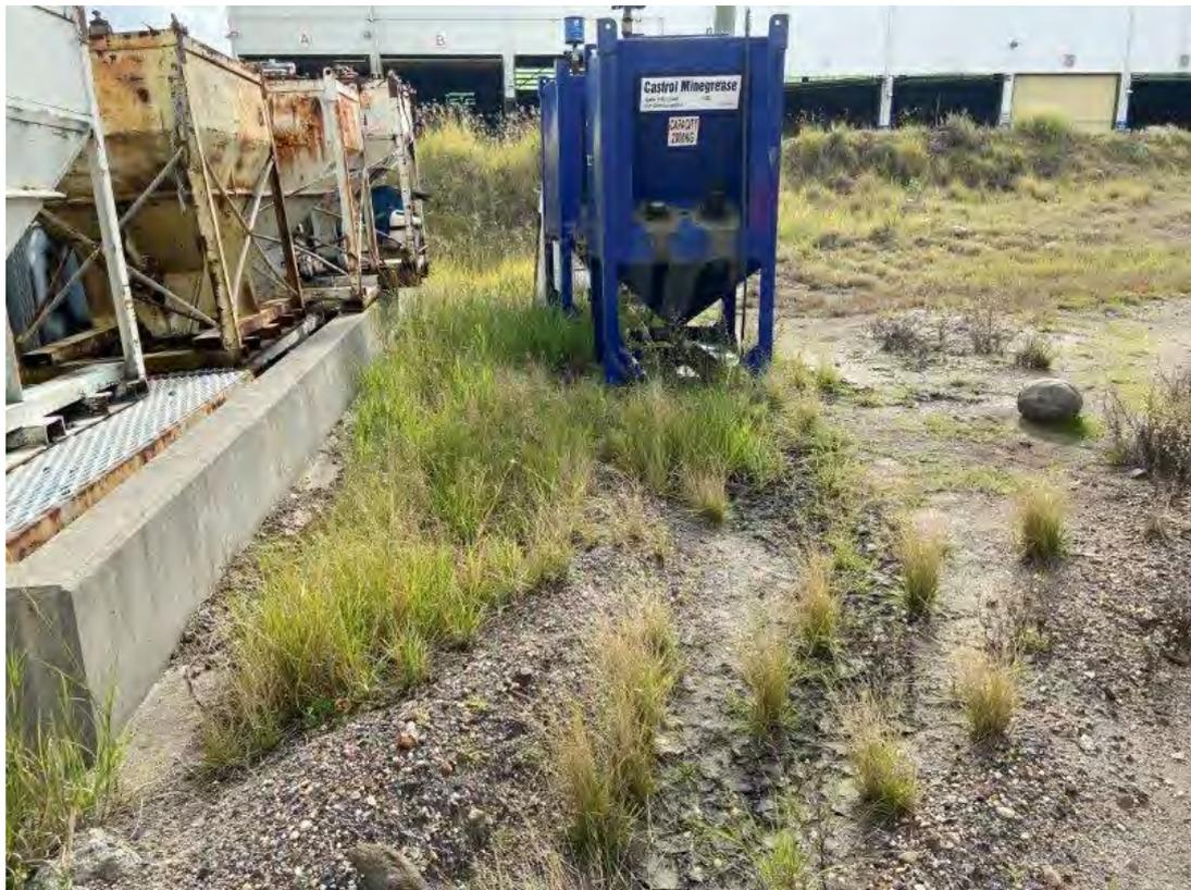
Plate 24 – Leaking fuel pod outside of bunded area
