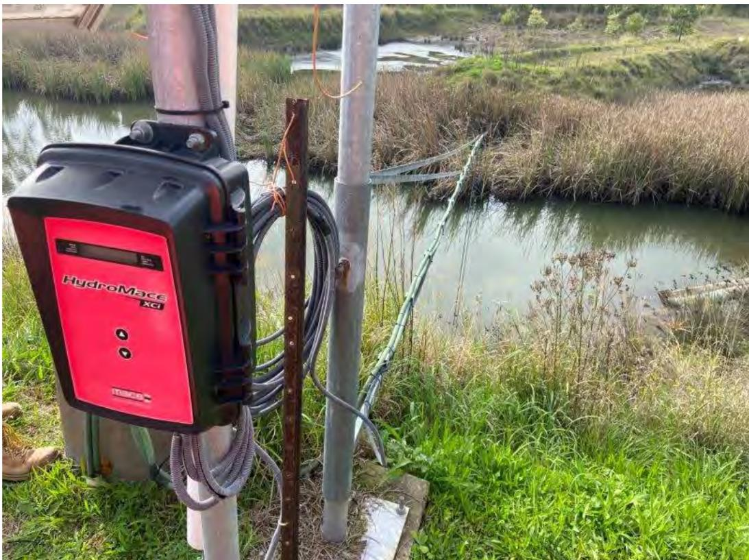
Plate 2 – Rail loop dam level indicator
