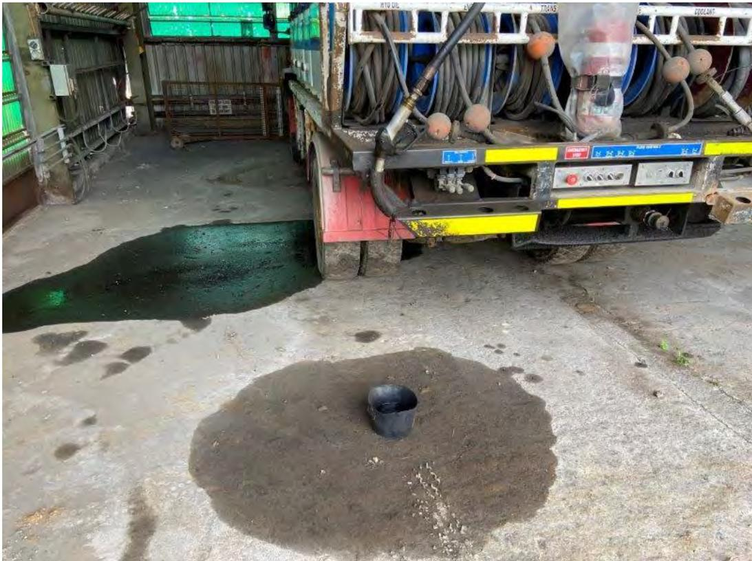
Plate 27 – Fuel and oil leaking from fuel cart during site inspection
