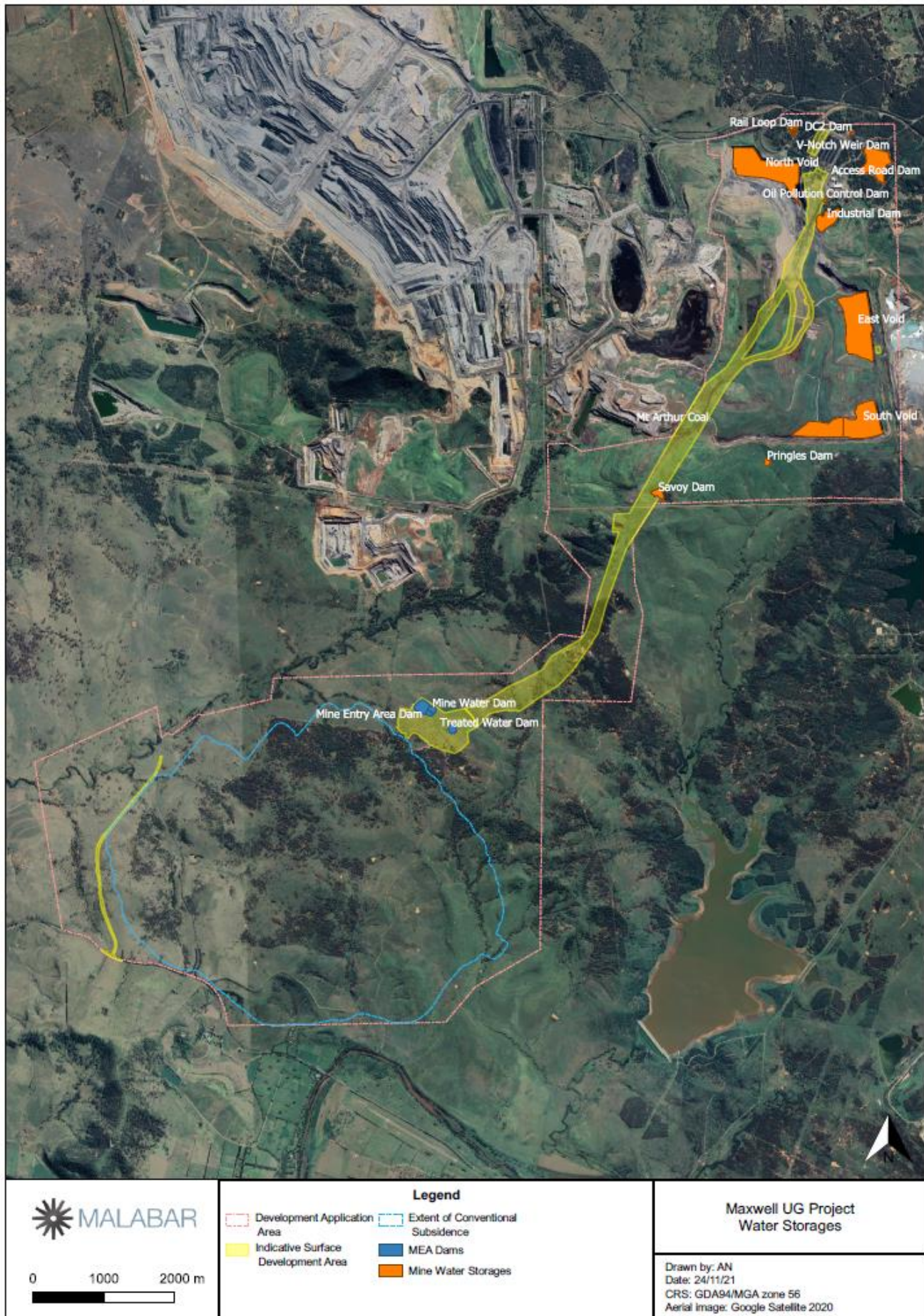
Figure 2: Existing and proposed mine water storages
