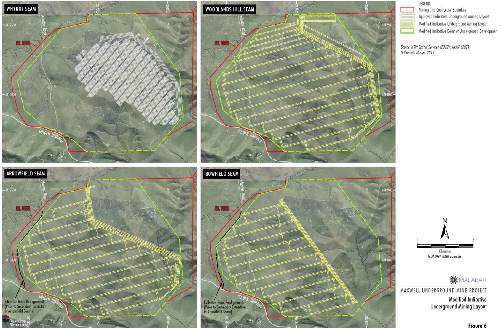
Figure 5 - Indicative Underground Mine Plan
