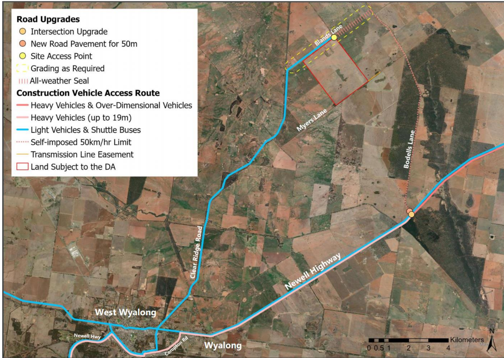
Figure 3 | Proposed road upgrades and site access
