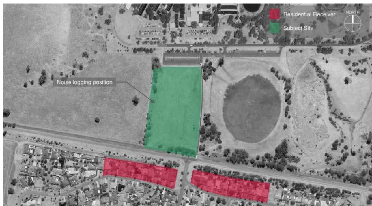
Figure 40 Noise monitoring and receiver locations
