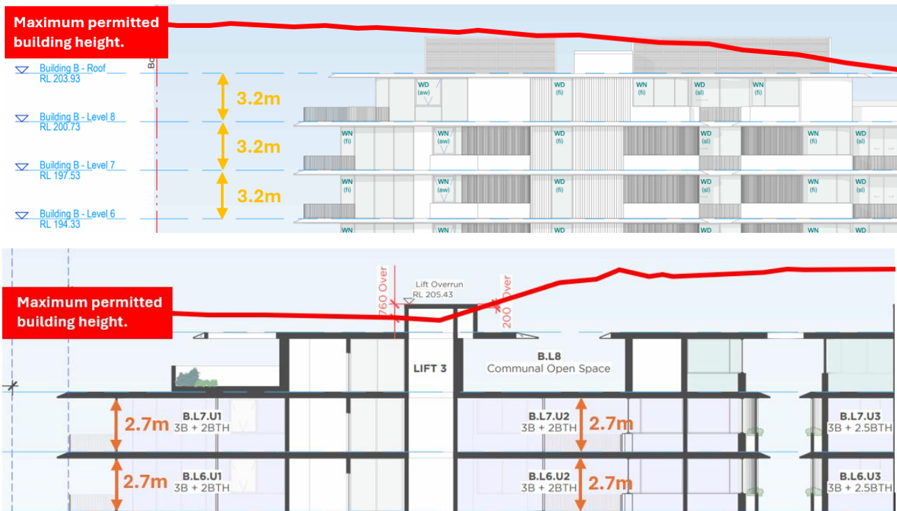
Figure 12 Extract: Proposed Slab Separation and Floor-to-Ceiling Heights
