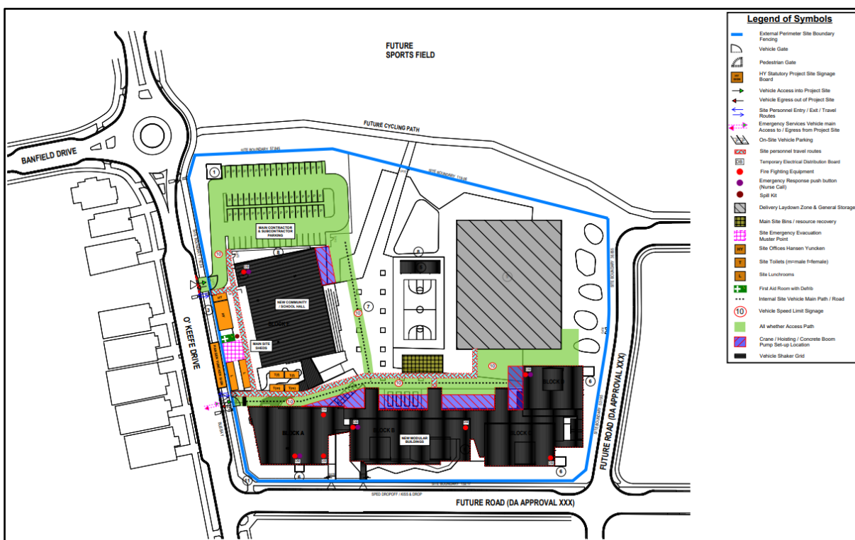
Figure 2: Construction Site Plan
