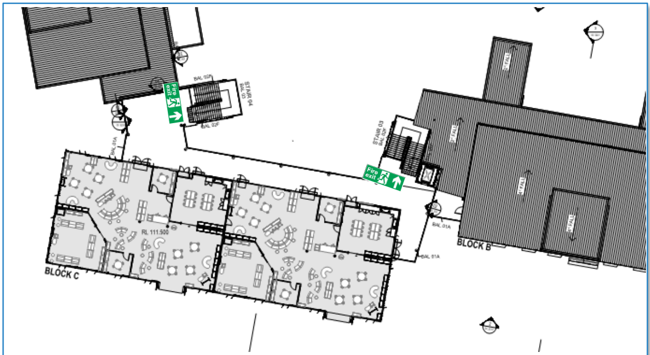
Figure 10: Exit provisions on Level 02 Block C
