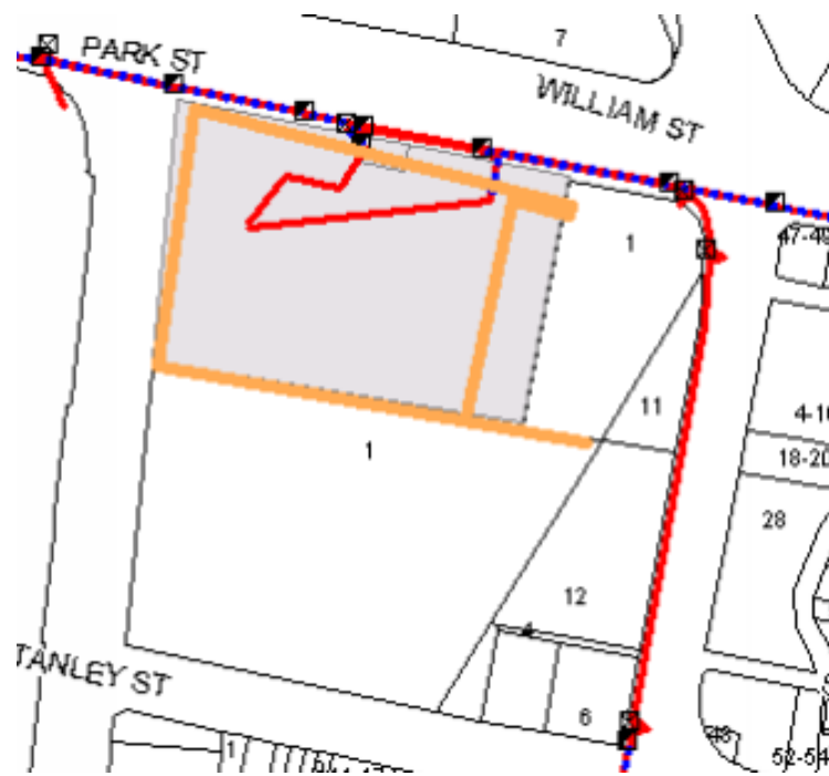
Figure 2: Existing Optus communications connection entering site William St
