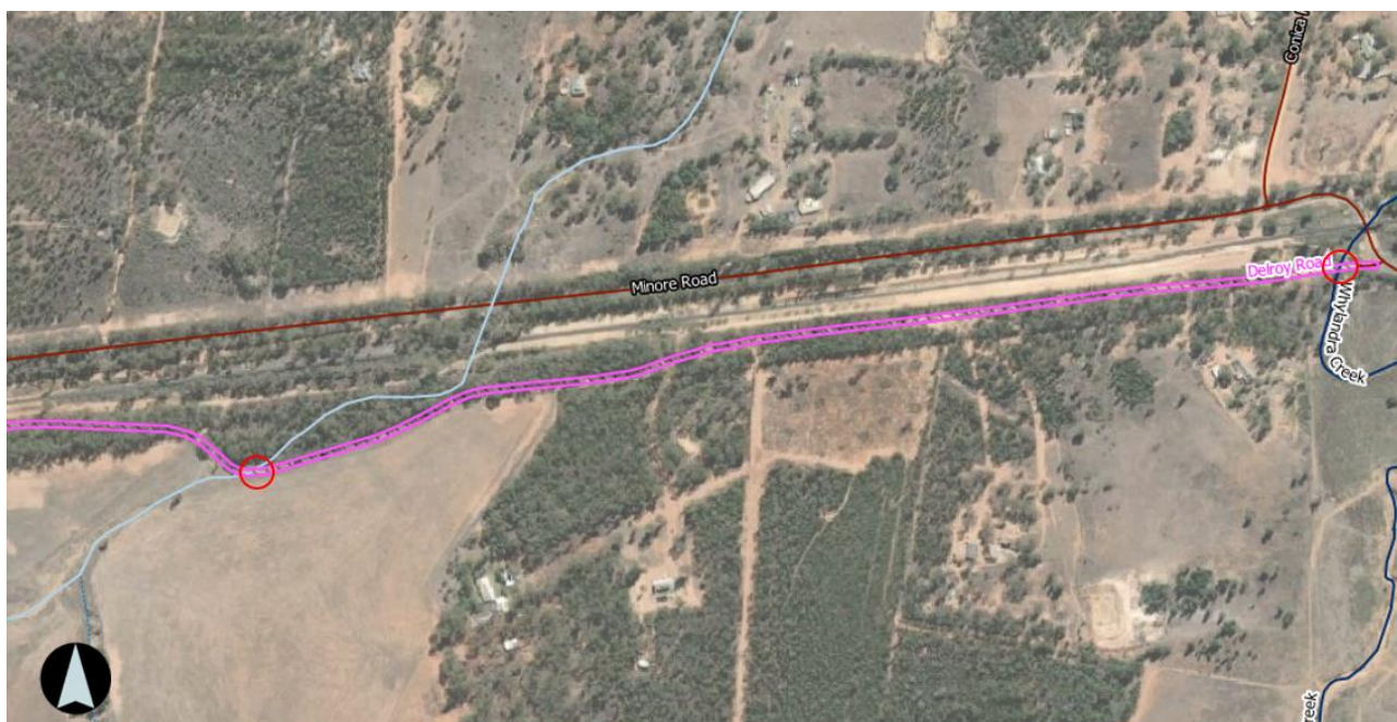
Figure 8-12 Potential flood points along Delroy Road (crossings indicated in red)
