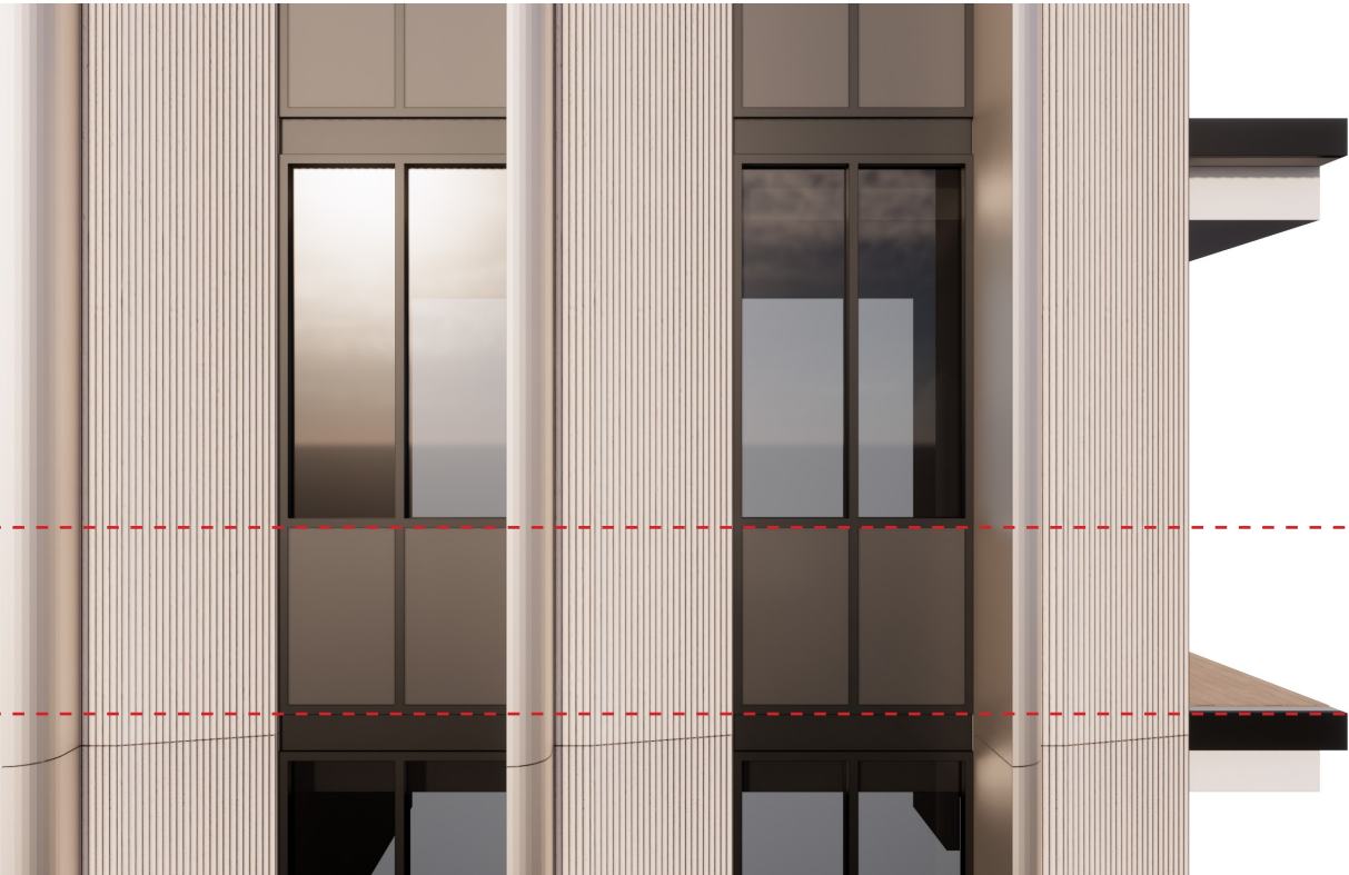
OPTION 02 - WITH 1m HIGH SPANDREL (2m ) - GLASS RATIO 45.1%
