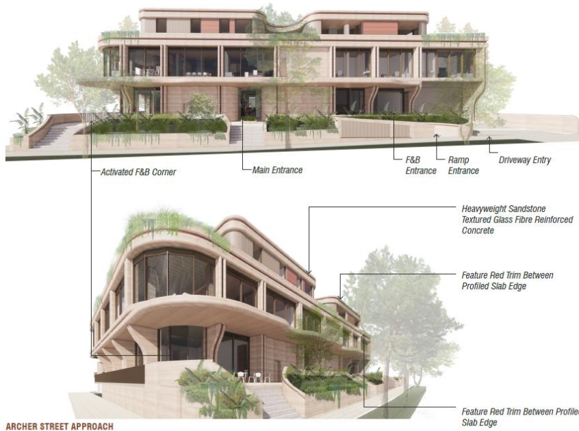
Figure 16 – Podium Façade Details Source: Team2
