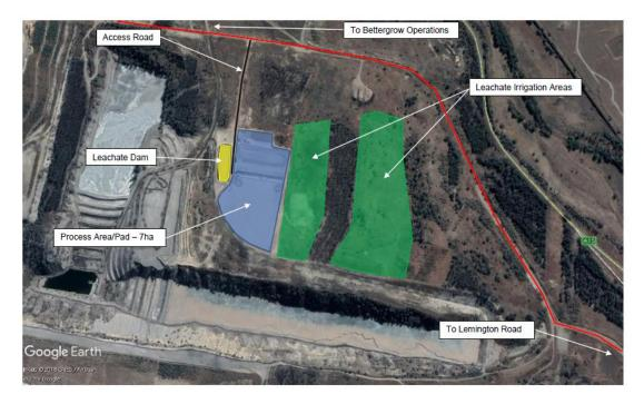
Figure 5: Layout of the Loop Organics Facility
