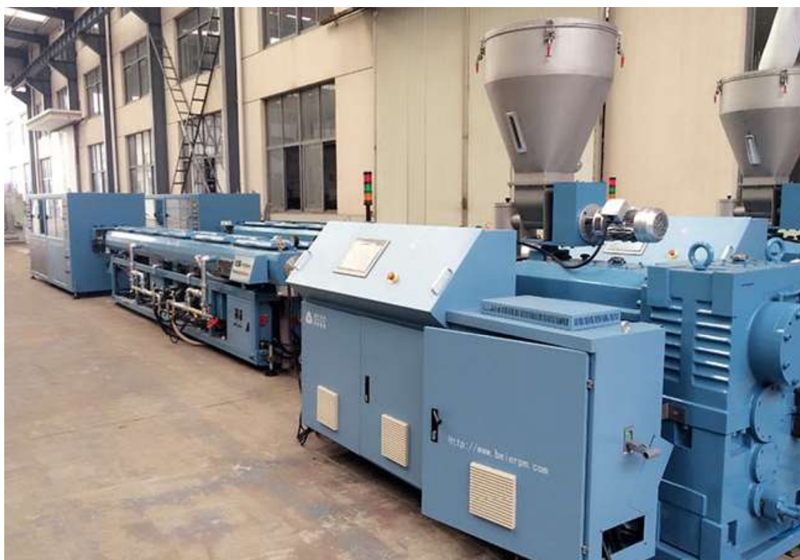
Figure 7.10 Example extrusion moulding production line for PE and PP pipes (Beier Machinery)
