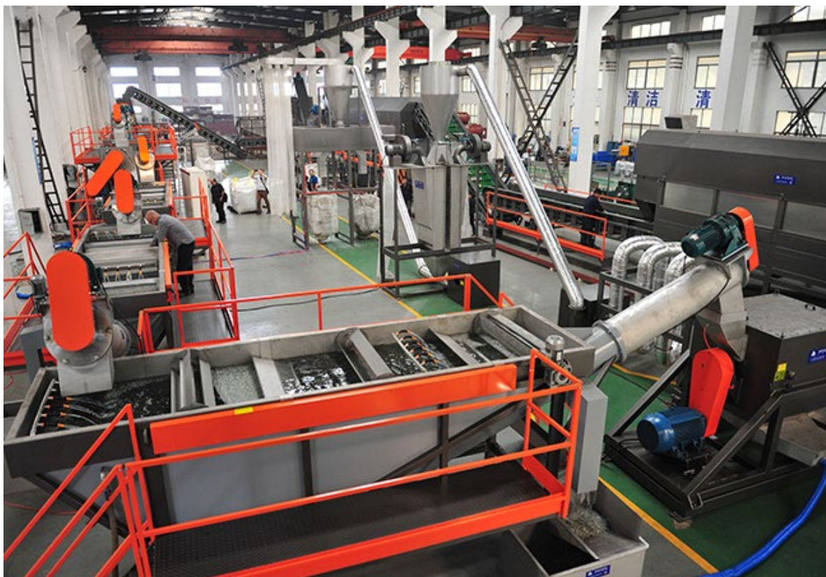
Figure 5.1 PET bottle washing and recycling lines (Beier Machinery)
