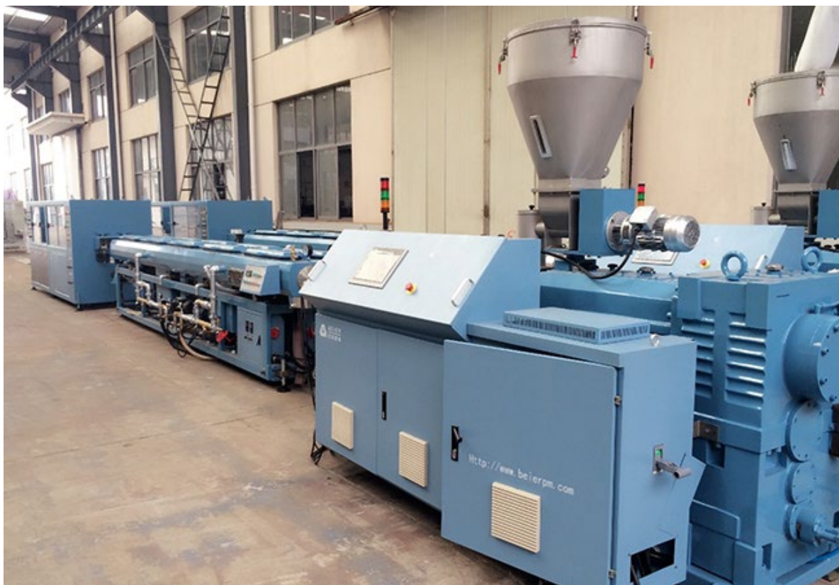
Figure 5.2 Extrusion moulding production line for PE and PP pipes (Beier Machinery)
