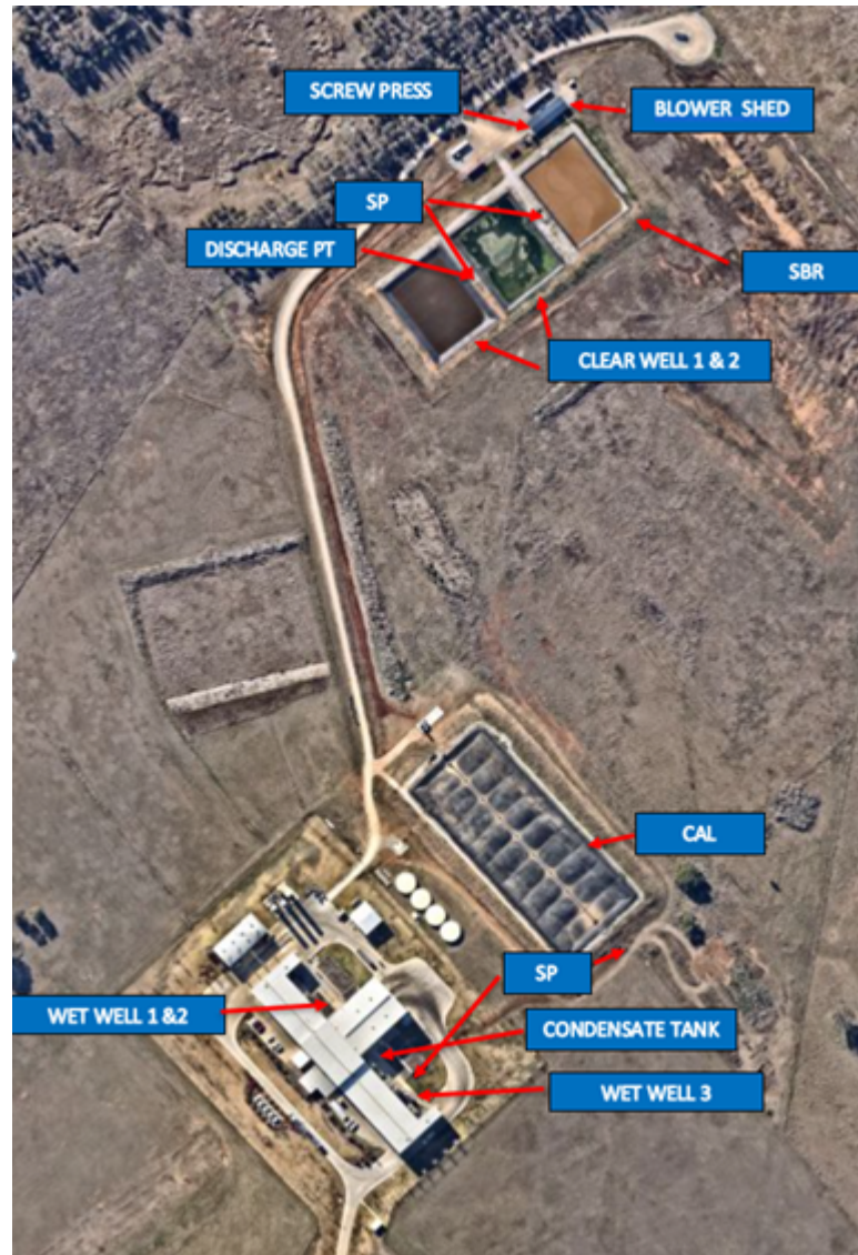
Figure 1 - Rendering Waste Water Key Infrastructure
