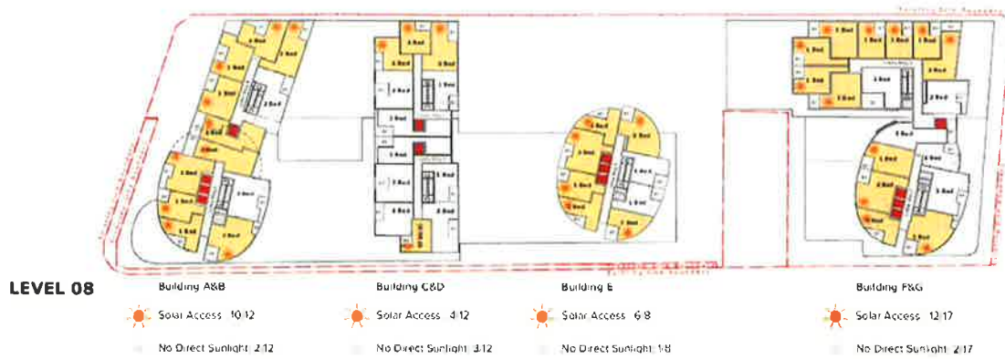
Figure 39 | Typical floor level of indicative scheme identifying a possible layout for residential uses in mid-rise and tower buildings and their solar access compliance
