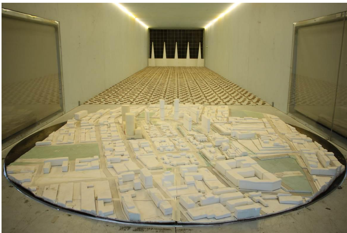
Figure 25: Photograph of the Wind Tunnel Model – (View from the South)
