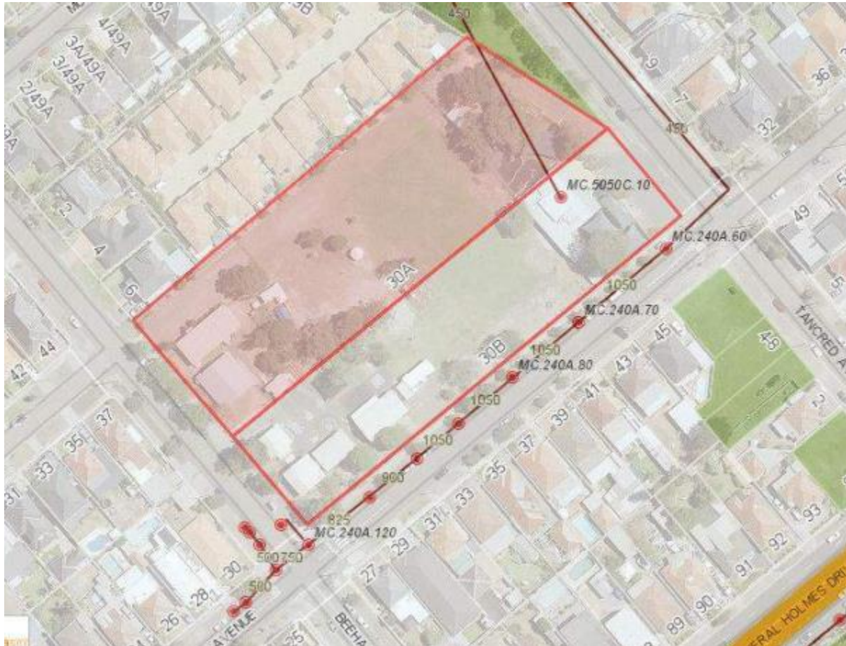
Figure 2.3.1 – Indicative External Stormwater system (Source: Bayside Council)
