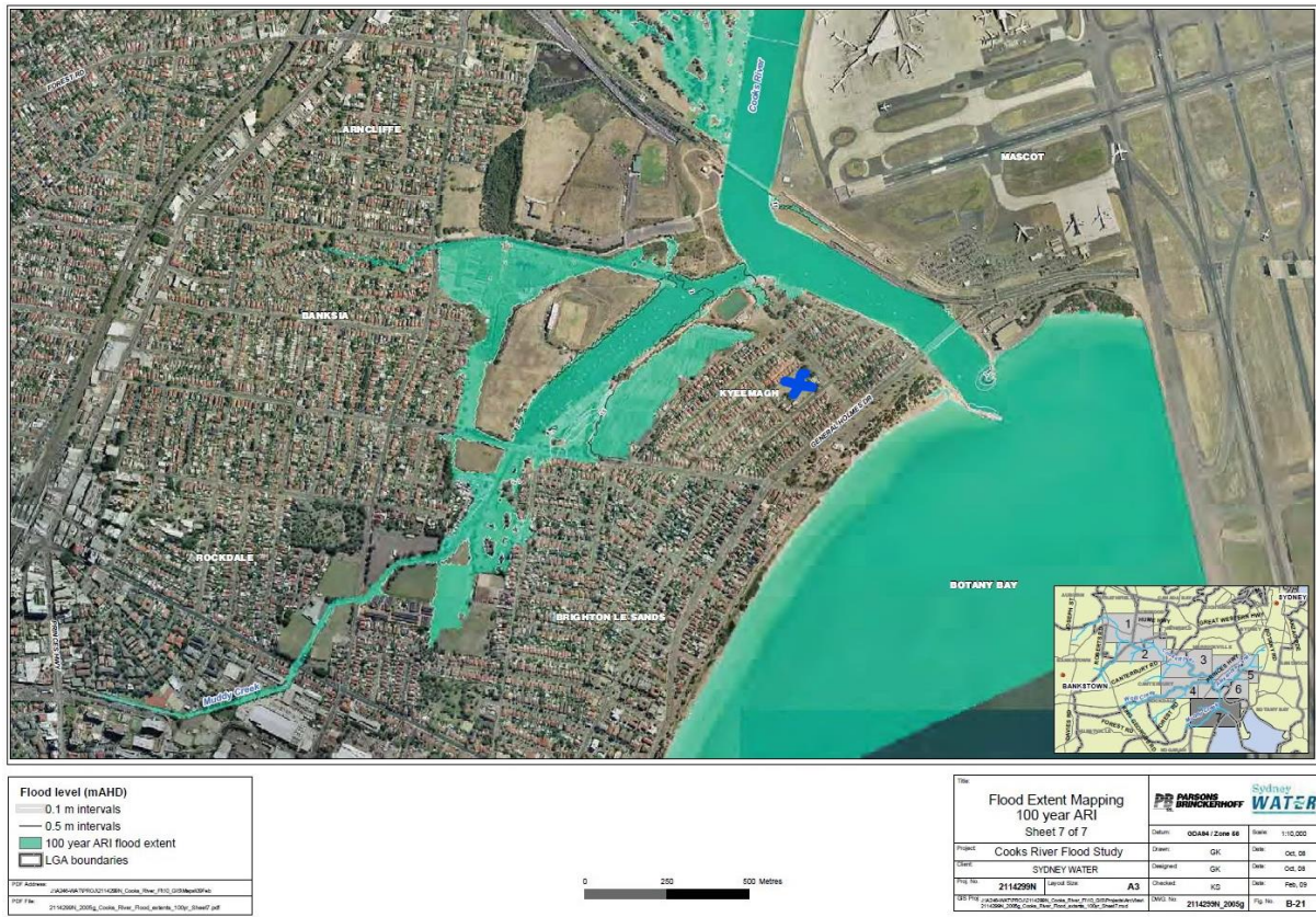
Figure 3.5.1 – Shows the 100 year flooding for Botany Bay & Cooks River (Source: Cardno)
