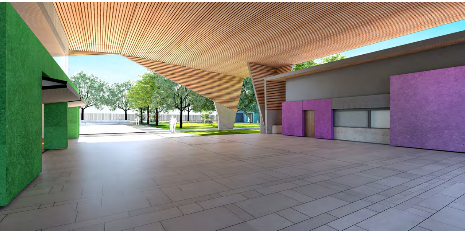
COLA ROOF ELEVATED TO BRING IN MORE LIGHT. ADDITIONAL CLEAR STORY LIGHTING ON NORTHERN FACADE. COLA IS OPEN TO DIRECT SUN FROM 3 SIDES - EAST / NORTH / WEST
