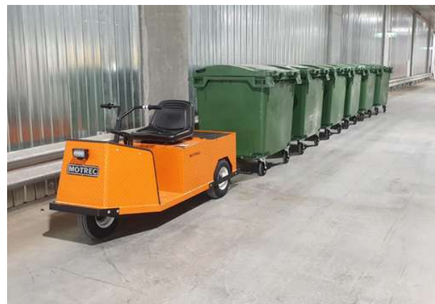
Application : Universal bin towing attachment attached to Motrec MP240 & 6x 1100ltr. waste bins
