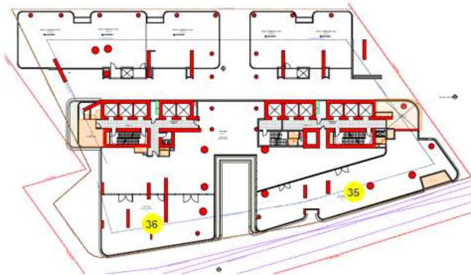
Figure 10 Sensor Locations on level 1- Proposed Scenario
