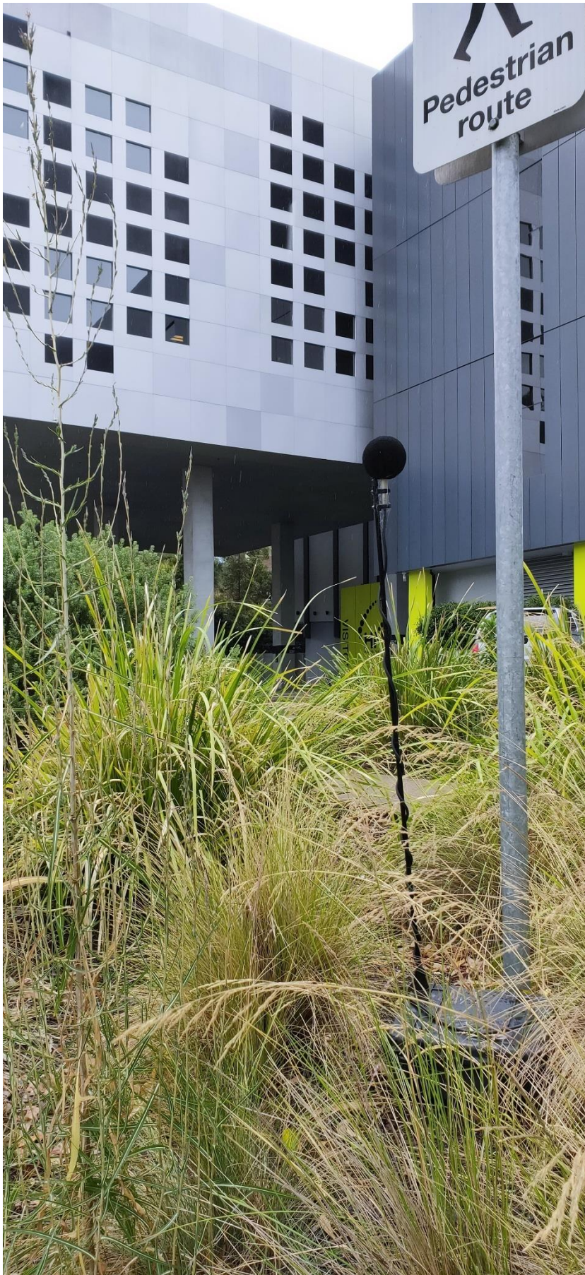
Photograph 7 – Noise monitor, HMRI building
