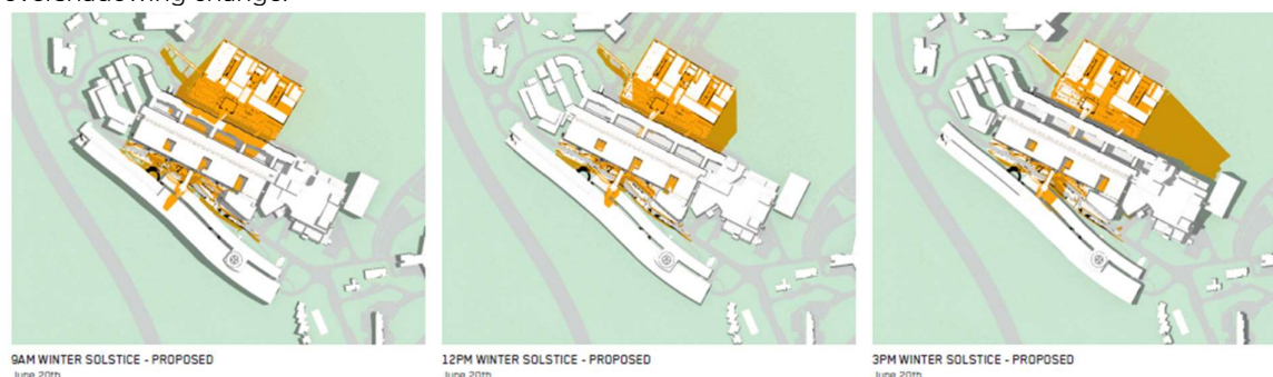
Figure 4 Revised solar diagrams for the winter solstice
