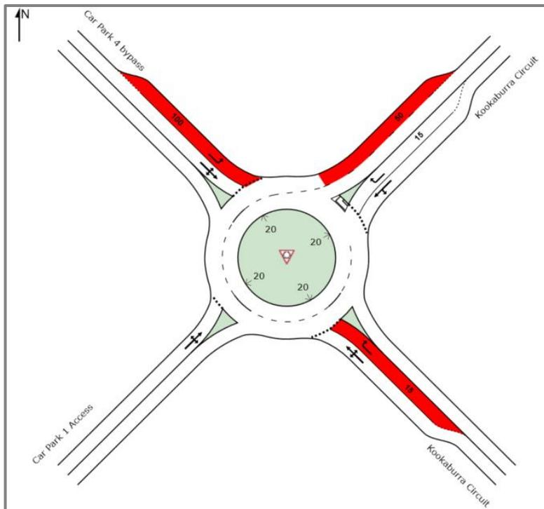
A swept path assessment has been completed confirming suitable access for NSW Fire Appliance vehicles to get to the ASB along the new northern road and Kookaburra Circuit via the two proposed roundabouts. The swept path assessment is provided in Appendix C.
