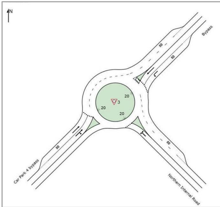
Figure 5.7: Proposed Roundabout Configuration (Kookaburra Circuit)
