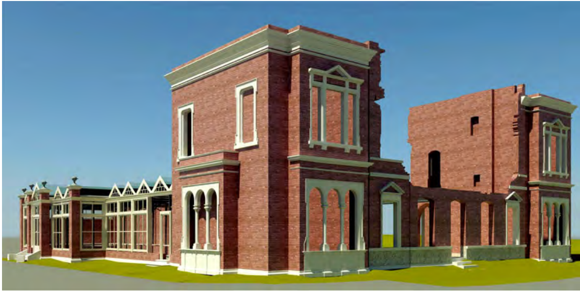
2: Woodseat Hall render output combining Point Cloud data to form the base BIM.
