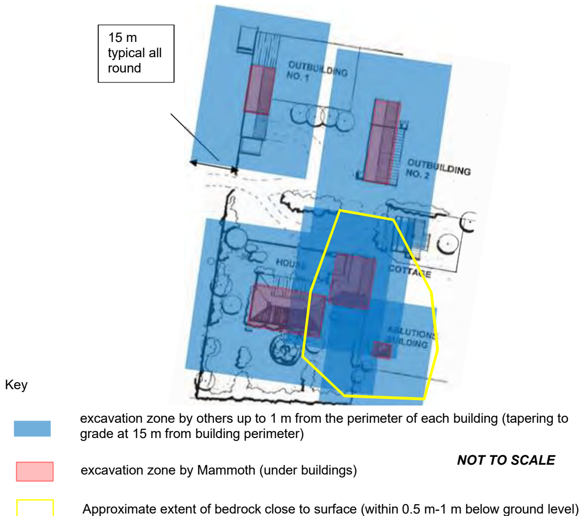
Figure 4 – Required excavation around buildings – plan view
