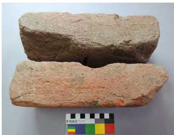
Figure 4.11: Worn sandstock rect shallow Rav bricks with fairly homogenous clay from TA4 TT03A, 55/#332 above 117/#335. Top left: stockface with frog. Top right: Strikeface with angled hackmarks to left. Lower left: side with lower 117/#335 having a slightly raised horizontal hackmark. Scale: 100mm. Photos: DSCN9754, 9759 and 9755.
