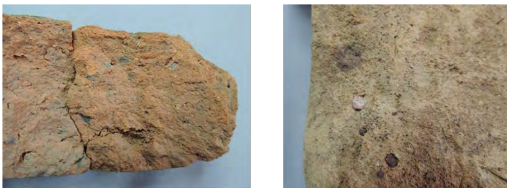
Figure 4.29: Clay fabric detail of sandstock rect shallow Rav bricks from TAs 4 and 6. Left: fired to a fairly homogenous deep red with grey ironstones and rare white quartz pebbles 126/#346. Right: fired to pink and white with red-brown ironstones and cracked white quartz pebbles 55/#328. Scale: 100mm. Photos: DSCN9844 and 9841.
