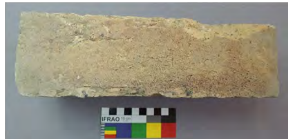
Figure 4.9: Sandstock rectangular Turton brick from TA3 TT6A, 2/#313 with stockface with 'TURTON' mark in rectangular frog, strikeface higher fired at right end, side with horizontal hackmark impressed during drying prior to firing. Scale: 100mm. Photos: DSCN9817, 9797, 9795 and 9802.
