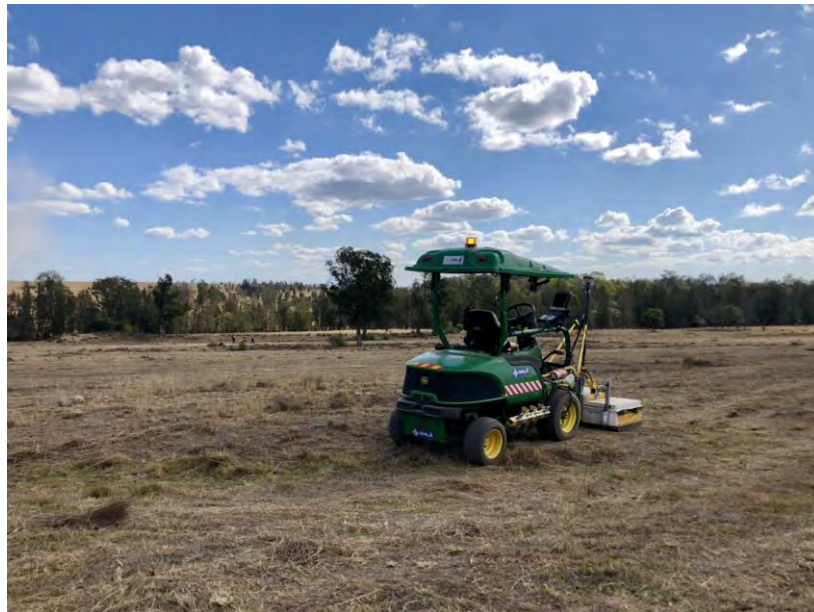
Figure 3: MALA 400MHz 3D MIRA acquiring data on site.
