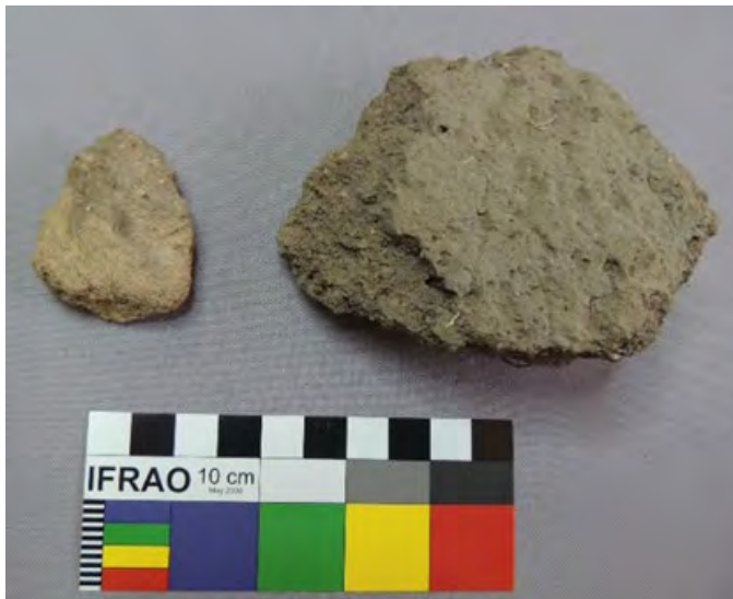
Figure 4.13: Dark grey-brown mud mortar samples from sandstone footings of potential convict barracks in Area 4. Left: TT3A 117/#339 (BM Sample 8). Right: TT5 35/#341 (BM Sample 5). Scale: 100mm. Photo: DSCN9849.
