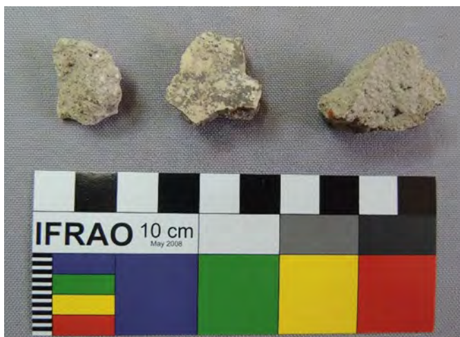
Figure 4.24: White-painted grey lime plaster render and set fragments from demolition rubble 133/#348 in TT8B in TA6. Scale: 100mm. Photo: DSCN9852.
