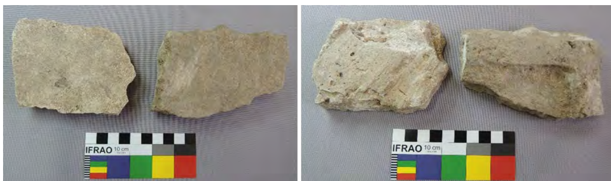
Figure 4.2: White to light grey render fragments from modified topsoil in TA3 TT2. Left: surface of two-coat lime plaster ceiling render #301 with slightly rough surface and two-coat wall render of harder smooth concrete set coat above lime plaster scratch/float coat. Right: underside of same fragments showing impressions of timber laths and wide joints of sandstone or brick masonry. Scale: 100mm. Photos: DSCN9855 and 9857.
