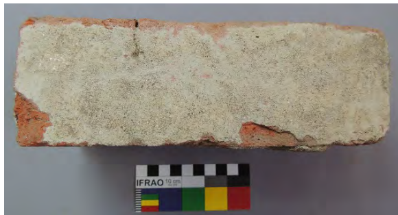
Figure 4.8: Sandstock rectangular narrow Rav brick from TA3 TT6A, 2/#311, three-quarter fragment. Top left: stockface with expanded clay beside large ironstone causing warping below frog. Top right: fairly smooth strikeface with red-brown ironstones and cream quartz. Lower left: one side with light grey-brown sandy lime mortar. Scale: 100mm. Photos: DSCN9814, 9785 and 9783.
