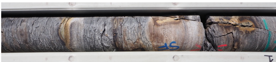
Plate 8 – Iron staining and sulphate salts due to partial oxidation of a pyritic zone. Hole GNC010, depth 22.00 to 22.45 m.
