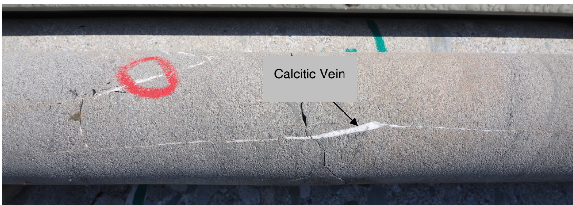
Plate 11 – Sandstone with calcitic carbonate in the matrix and veins. Hole GNC007, depth 67.8 m.
