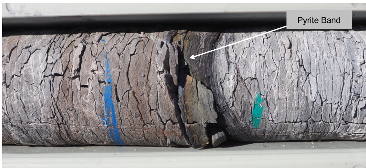
Plate 9 – Pyrite band (partly oxidised) parallel to bedding. Hole GNC007, depth 43.5 m.
