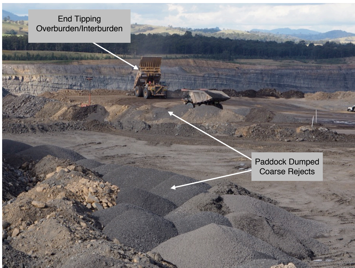
Plate 15 – End tipping of overburden/interburden and paddock dumping of coarse rejects in the Mount Owen North Pit.
