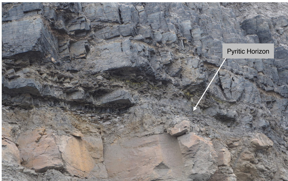
Plate 16 – Thin pyritic horizon on the Glendell Pit south wall, showing distinct yellow salts and iron staining due to pyrite oxidation.
