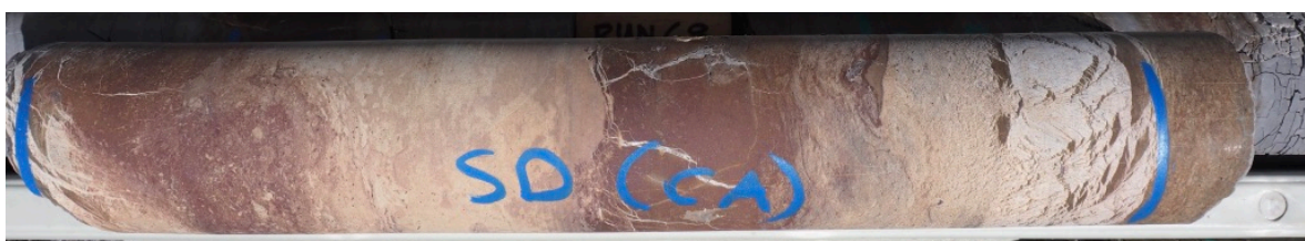
Plate 13 – Calcitic bands with cone-in-cone texture within a sideritic layer. Hole GNC010, depth 223.70 m.
