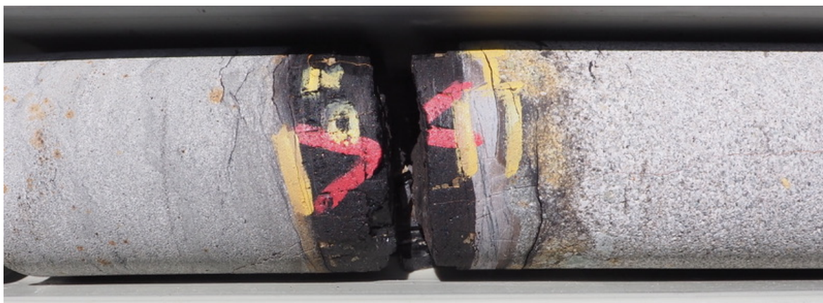
Plate 2 – Iron staining and sulphate salts due to partial oxidation of a pyrite coating parallel to bedding. Hole GNC010 68.30 m.
