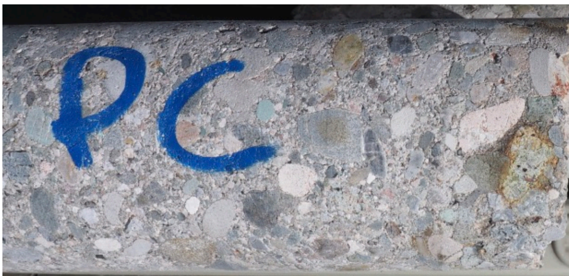
Plate 5 – Iron staining and sulphate salts due to partial oxidation of pyrite in a conglomerate clast. Hole GNC007, depth 103.00 m.
