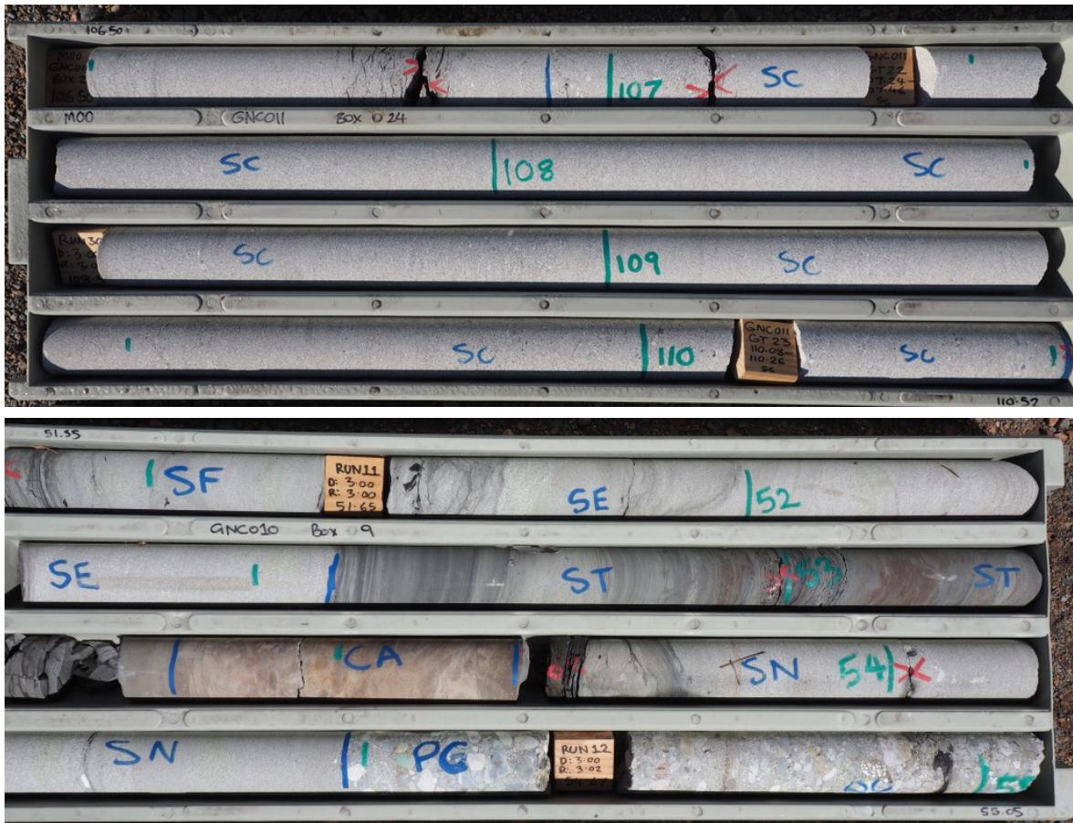
Plate 1 – Typical benign sandstone, and interbedded siltstone/sandstone/conglomerate overburden/interburden. Holes GNC011 depth 106.5 to 110.52 m (top), GNC010, depth 51.55 to 55.05 m (bottom).
