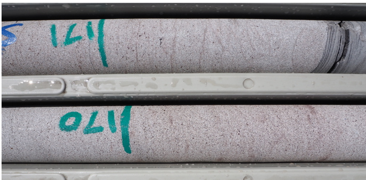
Plate 10 – Typical sandstone with calcitic carbonate in the matrix (shows reddish tinge). Hole GNC010, depth 168.35 to 177.25 m.
