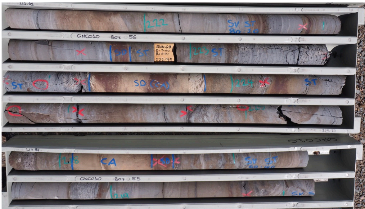
Plate 12 – Common siderite and calcitic lenses. Hole GNC010, depth 217.87 to 225.27 m.
