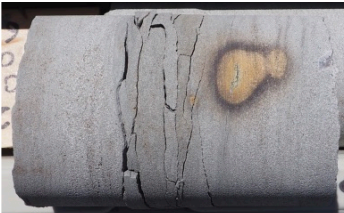
Plate 4 – Iron staining and sulphate salts due to partial oxidation of a pyrite containing lensoid in sandstone. Hole GNC010, depth 24.65 m.
