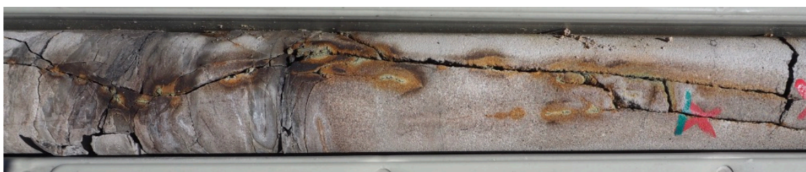
Plate 7 – Iron staining and sulphate salts due to partial oxidation of pyrite in a fracture. Hole GNC007, depth 45.4 m.
