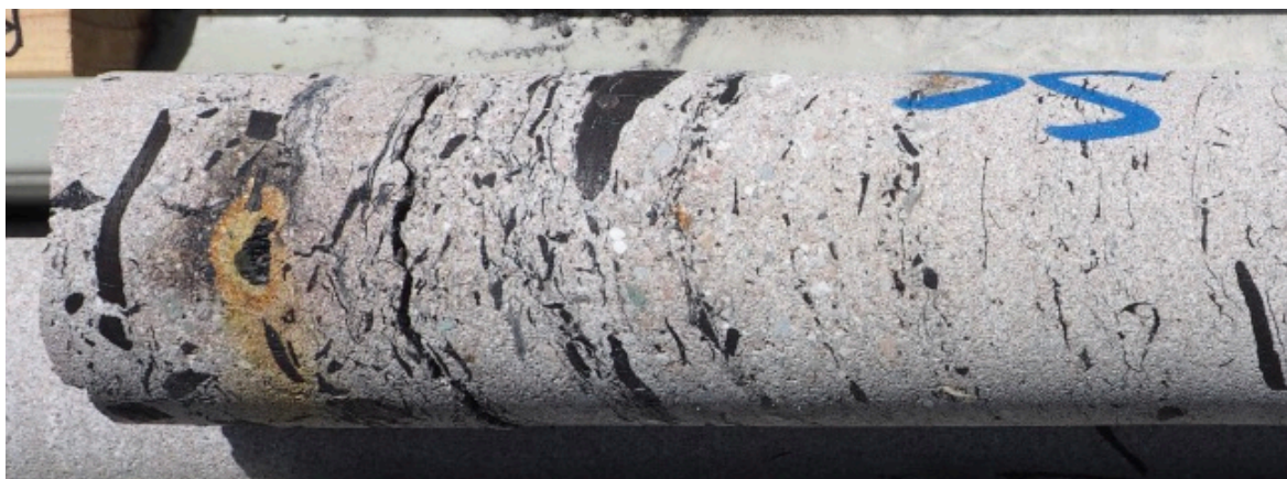
Plate 6 – Iron staining and sulphate salts due to partial oxidation of a pyrite associated with a carbonaceous wisp. Hole GNC010, depth 87.70 m.
