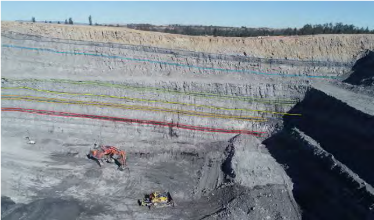
Figure 4-12 Glendell Pit western highwall showing the generally continuous nature of the coal seams
