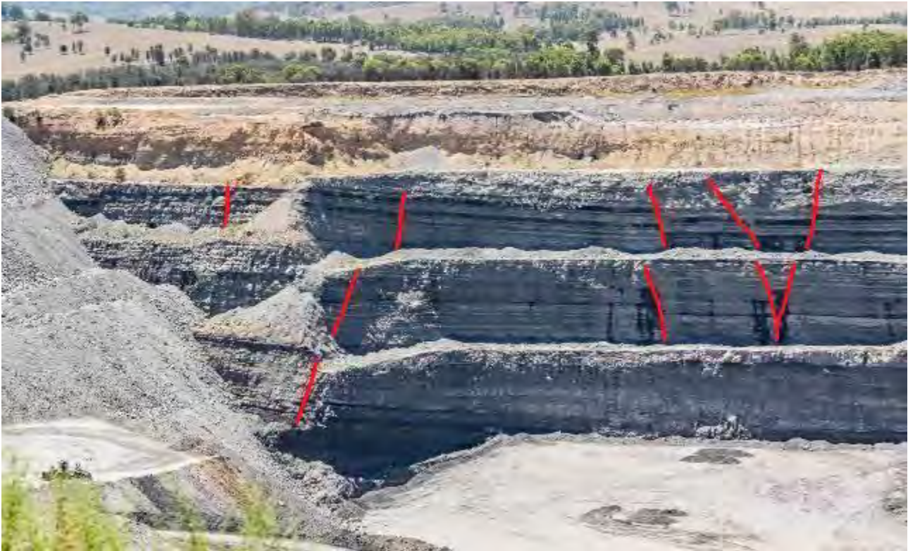
Figure 4-14 Block fault zone exposed at Bayswater North Pit (from PSM 2019)
