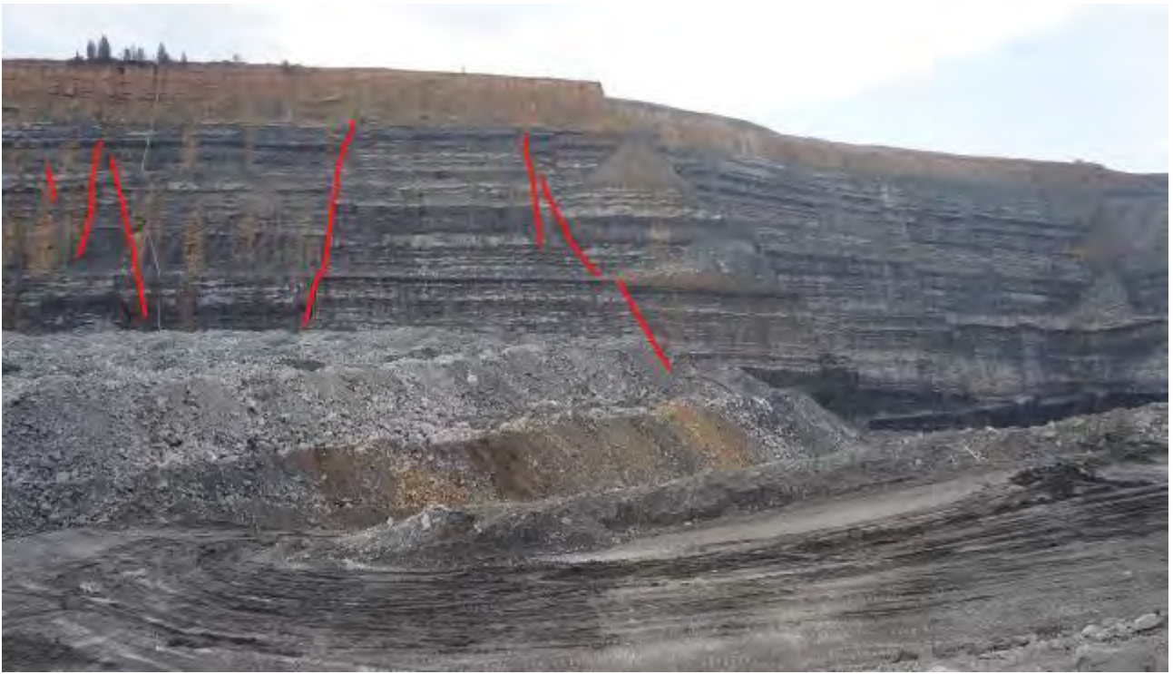
Figure 4-15 Block fault zone exposed at Bayswater North Pit in 2017 (from PSM 2019)
