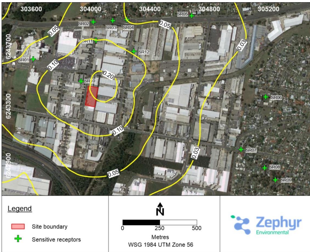
Figure 6-2: Predicted maximum 24-hour average PM_{2.5} concentration at the WTF ( \mu g/m^3 ) (Zephyr, 2022)
