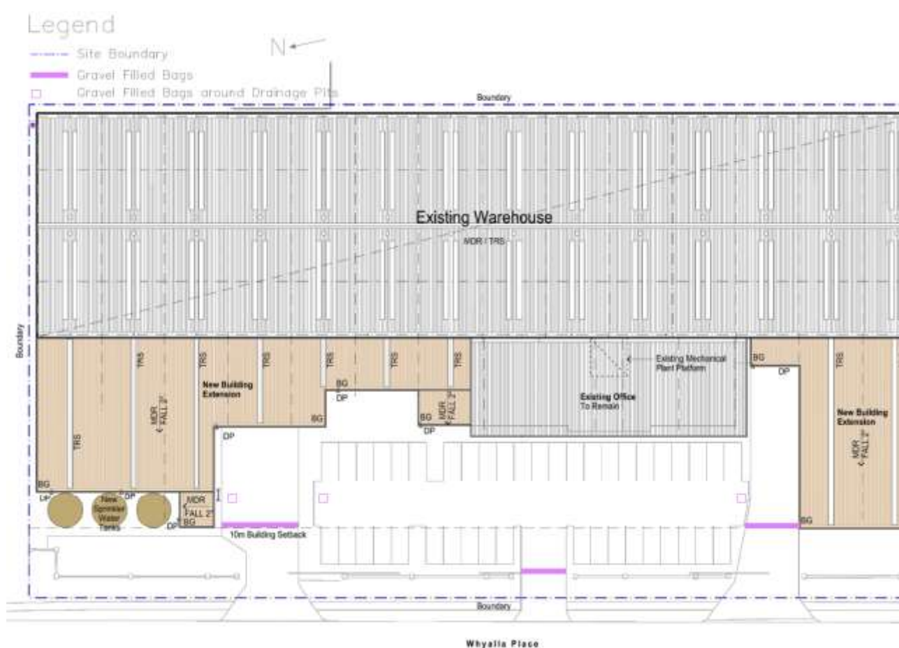
Figure 23: Erosion and sediment control plan (construction phase)
