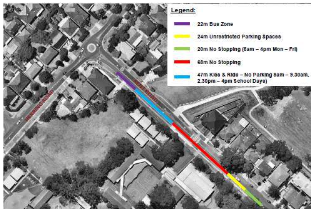
Figure 8 Existing set down / pick up arrangements
