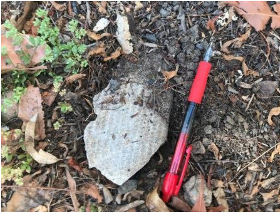
Image 6.6.1 Image of fibrous cement sheeting fragment in the vicinity of BH07
