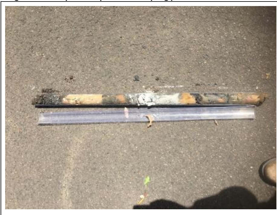
Image 6.2.1 Example of fill profile at sampling point BH32
