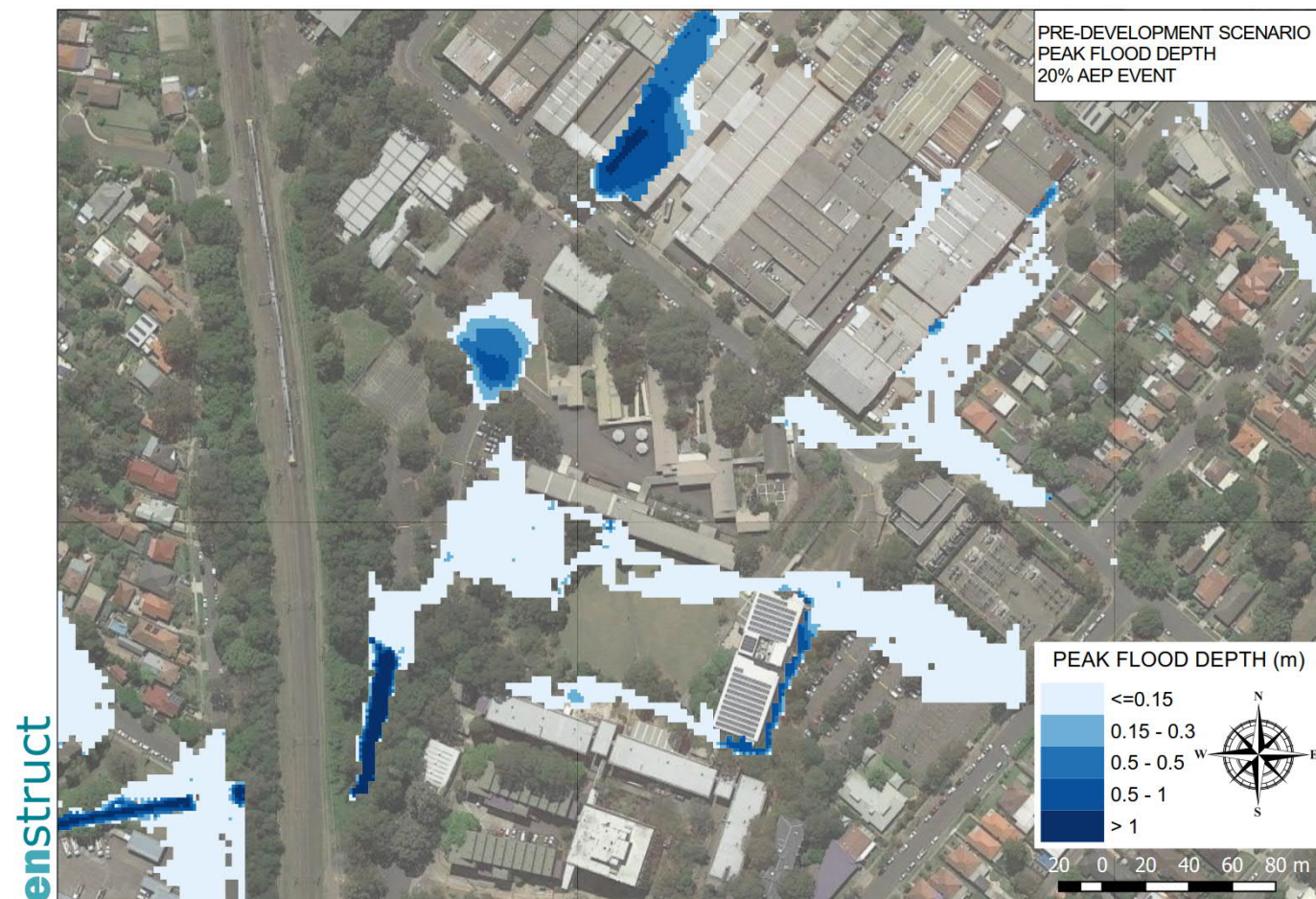
Figure 7. Overland flooding under existing conditions for 20% AEP event
